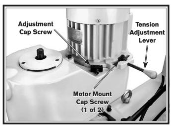
Figure 65. Belt tensioning controls.
